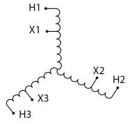
Three Phase Autotransformer with a capacity of 450kVA, transforming 550Y Volts to 400Y Volts
