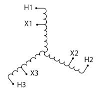
Three Phase Autotransformer with a capacity of 600kVA, transforming 230Y Volts to 550Y Volts
