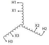
Three Phase Autotransformer with a capacity of 30kVA, transforming 200Y Volts to 277Y Volts
