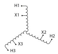
Three Phase Autotransformer with a capacity of 3kVA, transforming 200Y Volts to 277Y Volts
