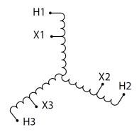
Three Phase Autotransformer with a capacity of 112.5kVA, transforming 380Y Volts to 115Y Volts
