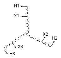
Three Phase Autotransformer with a capacity of 225kVA, transforming 120Y Volts to 230Y Volts
