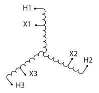
Three Phase Autotransformer with a capacity of 450kVA, transforming 120Y Volts to 460Y Volts
