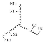
Three Phase Autotransformer with a capacity of 1000kVA, transforming 400Y Volts to 120Y Volts
