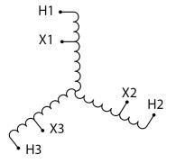
Three Phase Autotransformer with a capacity of 225kVA, transforming 550Y Volts to 277Y Volts
