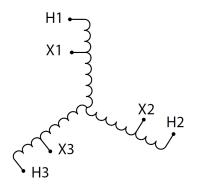
Three Phase Autotransformer with a capacity of 300kVA, transforming 460Y Volts to 380Y Volts
