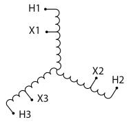
Three Phase Autotransformer with a capacity of 150kVA, transforming 550Y Volts to 200Y Volts
