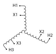
Three Phase Autotransformer with a capacity of 300kVA, transforming 200Y Volts to 400Y Volts
