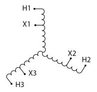
Three Phase Autotransformer with a capacity of 300kVA, transforming 347Y Volts to 400Y Volts
