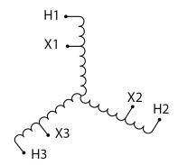
Three Phase Autotransformer with a capacity of 450kVA, transforming 380Y Volts to 600Y Volts
