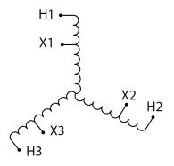
Three Phase Autotransformer with a capacity of 30kVA, transforming 220Y Volts to 400Y Volts
