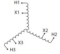
Three Phase Autotransformer with a capacity of 30kVA, transforming 600Y Volts to 400Y Volts
