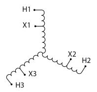
Three Phase Autotransformer with a capacity of 300kVA, transforming 600Y Volts to 415Y Volts
