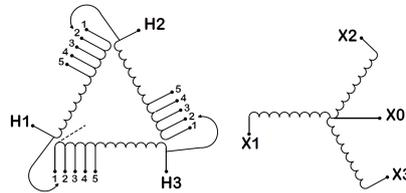
Three Phase Encapsulated Isolation Transformer with a capacity of 150kVA, transforming 460 Volts to 208Y/120 Volts
