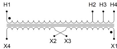
Single Phase Isolation Transformer with a capacity of 5kVA, transforming 460 Volts to 120/240 Volts
