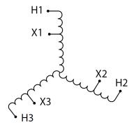
Three Phase Autotransformer with a capacity of 1500kVA, transforming 115Y Volts to 220Y Volts
