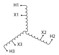
Three Phase Autotransformer with a capacity of 30kVA, transforming 220Y Volts to 460Y Volts
