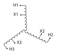
Three Phase Autotransformer with a capacity of 2500kVA, transforming 415Y Volts to 440Y Volts
