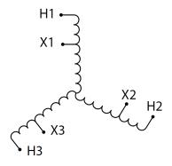
Three Phase Autotransformer with a capacity of 2500kVA, transforming 600Y Volts to 440Y Volts
