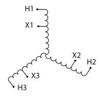
Three Phase Autotransformer with a capacity of 600kVA, transforming 416Y Volts to 110Y Volts
