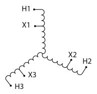
Three Phase Autotransformer with a capacity of 2500kVA, transforming 415Y Volts to 460Y Volts
