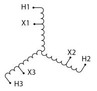
Three Phase Autotransformer with a capacity of 1500kVA, transforming 400Y Volts to 277Y Volts
