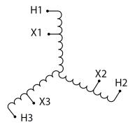
Three Phase Autotransformer with a capacity of 1500kVA, transforming 550Y Volts to 277Y Volts
