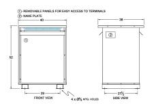
Three Phase Isolation Transformer with a capacity of 225kVA, transforming 240 Volts to 416Y/240 Volts
