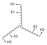
Three Phase Autotransformer with a capacity of 30kVA, transforming 220Y Volts to 575Y Volts
