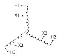
Three Phase Autotransformer with a capacity of 225kVA, transforming 600Y Volts to 460Y Volts
