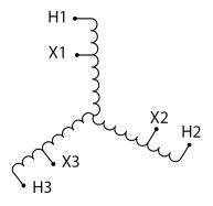
Three Phase Autotransformer with a capacity of 2000kVA, transforming 600Y Volts to 415Y Volts
