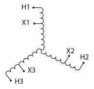
Three Phase Autotransformer with a capacity of 1000kVA, transforming 550Y Volts to 208Y Volts
