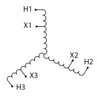
Three Phase Autotransformer with a capacity of 500kVA, transforming 600Y Volts to 115Y Volts
