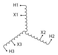
Three Phase Autotransformer with a capacity of 150kVA, transforming 400Y Volts to 347Y Volts
