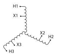
Three Phase Autotransformer with a capacity of 500kVA, transforming 400Y Volts to 120Y Volts
