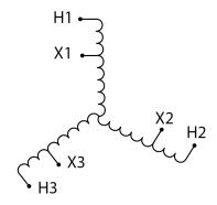
Three Phase Autotransformer with a capacity of 2000kVA, transforming 400Y Volts to 480Y Volts
