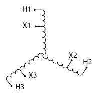
Three Phase Autotransformer with a capacity of 2500kVA, transforming 575Y Volts to 600Y Volts
