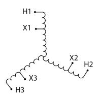
Three Phase Autotransformer with a capacity of 45kVA, transforming 380Y Volts to 110Y Volts
