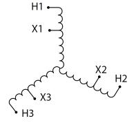
Three Phase Autotransformer with a capacity of 15kVA, transforming 575Y Volts to 380Y Volts
