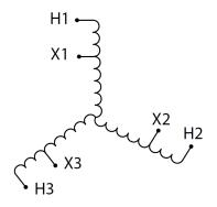
Three Phase Autotransformer with a capacity of 450kVA, transforming 400Y Volts to 120Y Volts
