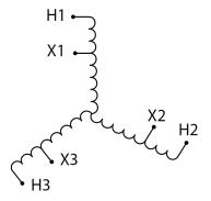
Three Phase Autotransformer with a capacity of 1500kVA, transforming 600Y Volts to 400Y Volts
