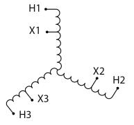
Three Phase Autotransformer with a capacity of 225kVA, transforming 200Y Volts to 600Y Volts
