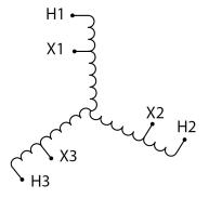
Three Phase Autotransformer with a capacity of 1500kVA, transforming 600Y Volts to 415Y Volts
