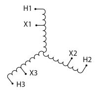
Three Phase Autotransformer with a capacity of 150kVA, transforming 230Y Volts to 415Y Volts
