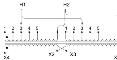
Single Phase Isolation Transformer with a capacity of 75kVA, transforming 600 Volts to 380 Volts
