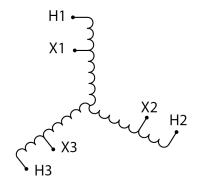
Three Phase Autotransformer with a capacity of 600kVA, transforming 416Y Volts to 200Y Volts
