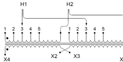
Single Phase Isolation Transformer with a capacity of 37.5kVA, transforming 380 Volts to 220 Volts
