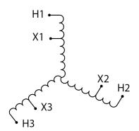
Three Phase Autotransformer with a capacity of 600kVA, transforming 600Y Volts to 208Y Volts
