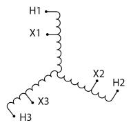
Three Phase Autotransformer with a capacity of 300kVA, transforming 416Y Volts to 110Y Volts
