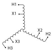
Three Phase Autotransformer with a capacity of 600kVA, transforming 415Y Volts to 220Y Volts
